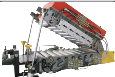
Standard - 11 straightening rolls
