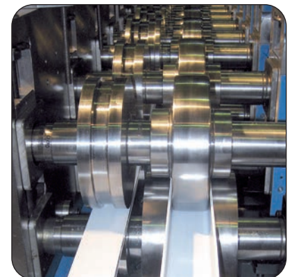
Simultaneous rollforming of 2 parts
