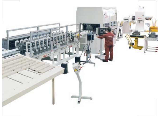
Production line of fluorescent battens
