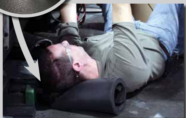
Lock the mat in the rolled position using the 2 connectors to obtain support for the neck and head.
