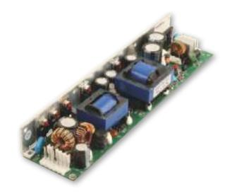
whatever reason, they need to be powered by the DC bus and changeover is to be effected without interruption. This is a particular feature designed by Powerbox in the OFMA60AD12, thus guaranteeing full performance in both conditions.
