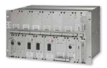
The power supplies units are enclosed in metal cases with a 230Vac input, delivering regulated voltage to the signaling equipment (ac and dc). The system also incorporates a power supply backup system based around SLA batteries.
