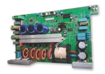
An automatic current controller guarantees that the power envelope is always within safe limits, reducing capacitor aging and overstressing of components, thus contributing to a longer lifetime. The SMM3000A80024-C has a built-in microprocessor constantly monitoring the charging status, reporting end of charge and discharge level, as well as all protection warnings due to abnormal operation such as over-temperature, over-voltage and current.
