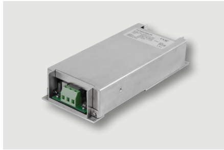
Defense line 300 300W, Enclosed, rugged design AC/DC switch mode power supply 85-264VAC input with PFC 1-2 isolated outputs
