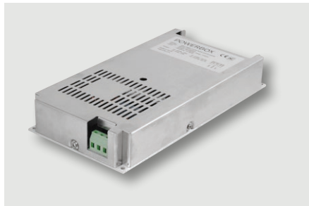
Defense line 1200 1200W, Enclosed, rugged design AC/DC switch mode power supply 85-264VAC or 120-350VDC input voltage 1-6 isolated outputs
