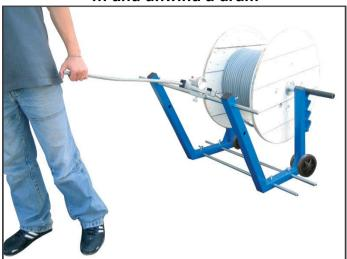
Very flexible unwinding thanks to the aluminum centering devices (78 mm Ø), which rotate around a steel shaft (Ø 35 mm) An additional shaft + 2 centering pin set, supplied with the device, can be ordered in order to preequip other drums and therefore make the loading process faster (code ST1-ST2-XAXE)
