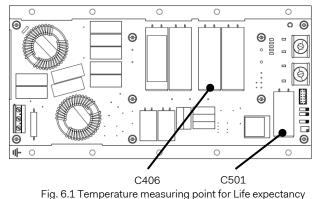
rig. 0.1 remperature measuring point for Life ex
