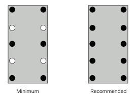
Fig. 1.1 Mounting hole requirement
