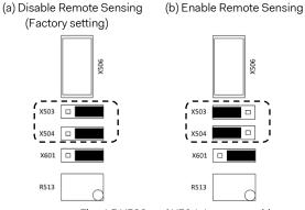
Fig. 4.5 X503 and X504 Jumper position
