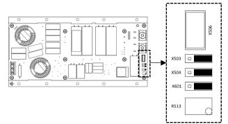
Fig. 3.2 Jumper placement at factory
