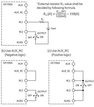
Fig. 4.4 Example of connecting remote ON/OFF circuit
