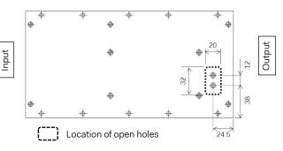
Fig. 1.2 Location of open hole on Aluminum Baseplate (Bottom view)
