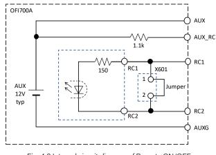
Fig. 4.3 Internal circuit diagram of Remote ON/OFF
