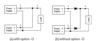
Fig. 5.2 example of 1+1 Redundancy operation
