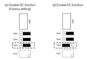
Fig. 4.2 X601 Jumper position
