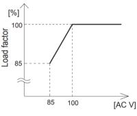
Fig. 2.1 Derating curve by input voltage
