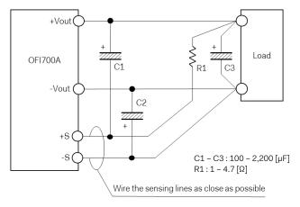
Fig. 4.6 When using remote sensing function
