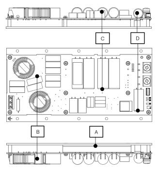
Fig. 2.2 Temperature measuring points
