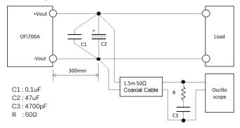
Fig.3.3 Method of Measuring Output ripple and ripple noise
