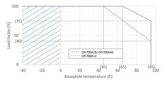
Fig. 2.3 Derating curve of point A (baseplate temperature)
