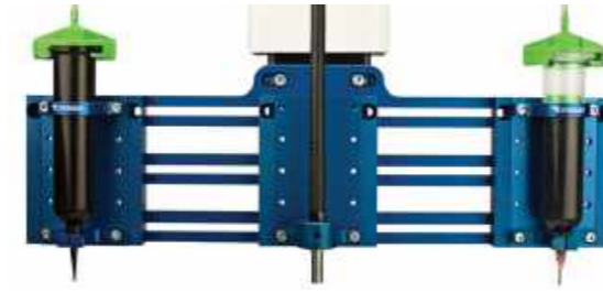
Example configuration dual syringe and light guide.
